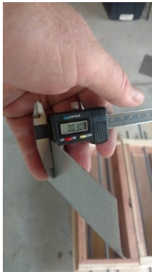
Exhibit showing 0.03" (1/32") shim placed mid-point across specimen for 4 hours and removed.
