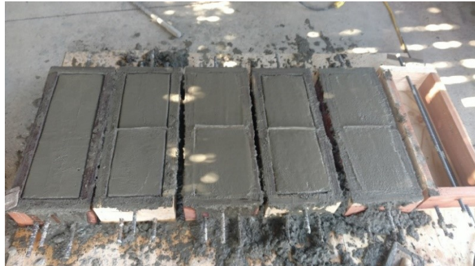
Exhibit showing 0.03" (1/32") shim placed mid-point across specimen for 4 hours and removed.
