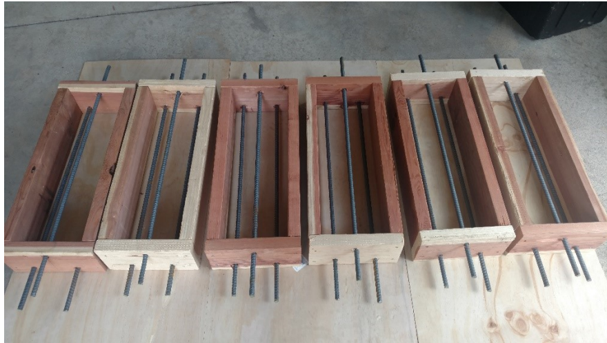
Exhibits showing specimen size and rebar layout.
